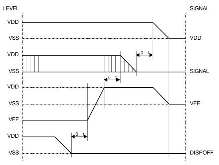
Please maintain the above sequence when turning on and off the power supply of the module. If DISPOFF is supplied to the module while internal alternate signal for LCD driving (M) is unstable, DC component will be supplied to the LCD panel. This may cause damage the LCD module.
