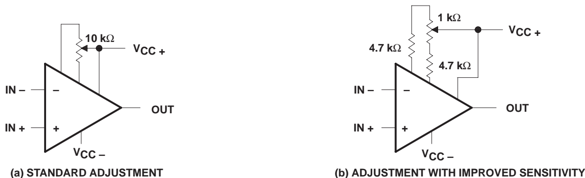
Figure 55. Input Offset Voltage Nulling Circuits
