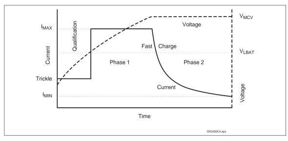
Figure 3. Lithium-Ion Charge Algorithm
