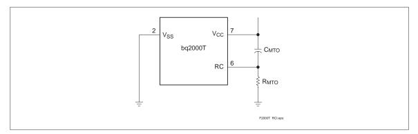
Figure 4. Typical Connection for the RC Input
