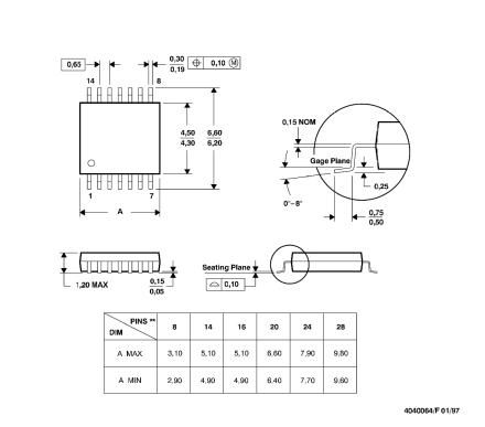
NOTES: A. All linear dimensions are in millimeters. B. This drawing is subject to change without notice. C. Body dimensions do not include mold flash or protrusion not to exceed 0,15. D. Falls within JEDEC MO-153
