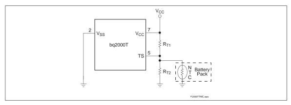
Figure 5. Temperature Monitoring Configuration
