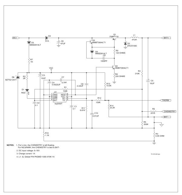
Figure 8. Single-Cell Li-Ion, Three-Cell NiCd/NiMH 1A Charger
