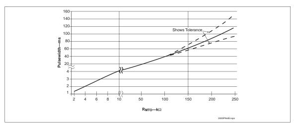
Figure 7. Relationship Between Trickle Pulse-Width and Value of R<sub>MTO</sub>
