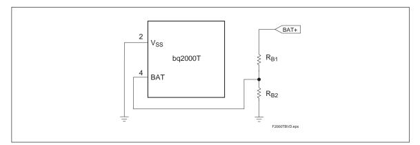
Figure 6. Battery Voltage Divider
