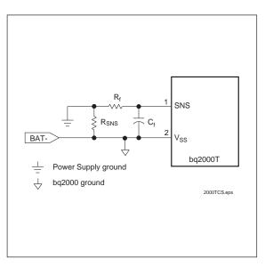
Figure 9. Current-Sensing Circuit
