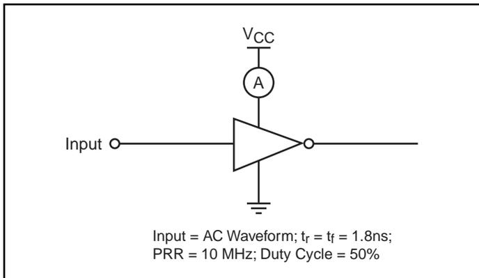
Figure 2. I<sub>CCD</sub> Test Circuit
