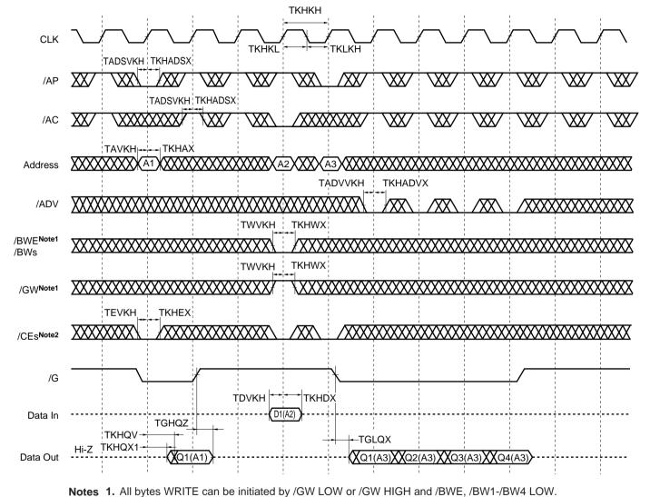
2. /CEs refers to /CE, CE2 and /CE2. When /CEs is LOW, /CE and /CE2 are LOW and CE2 is HIGH. When /CEs is HIGH, /CE and /CE2 are HIGH and CE2 is LOW.
