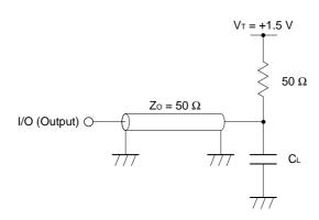
**Remark** CL includes capacitances of the probe and jig, and stray capacitances.
