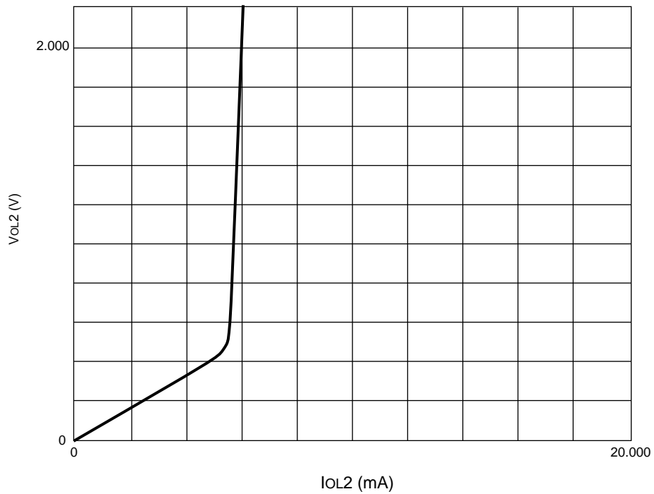
“L” Level Output Current vs. “L” Level Output Voltage (PLL2)
