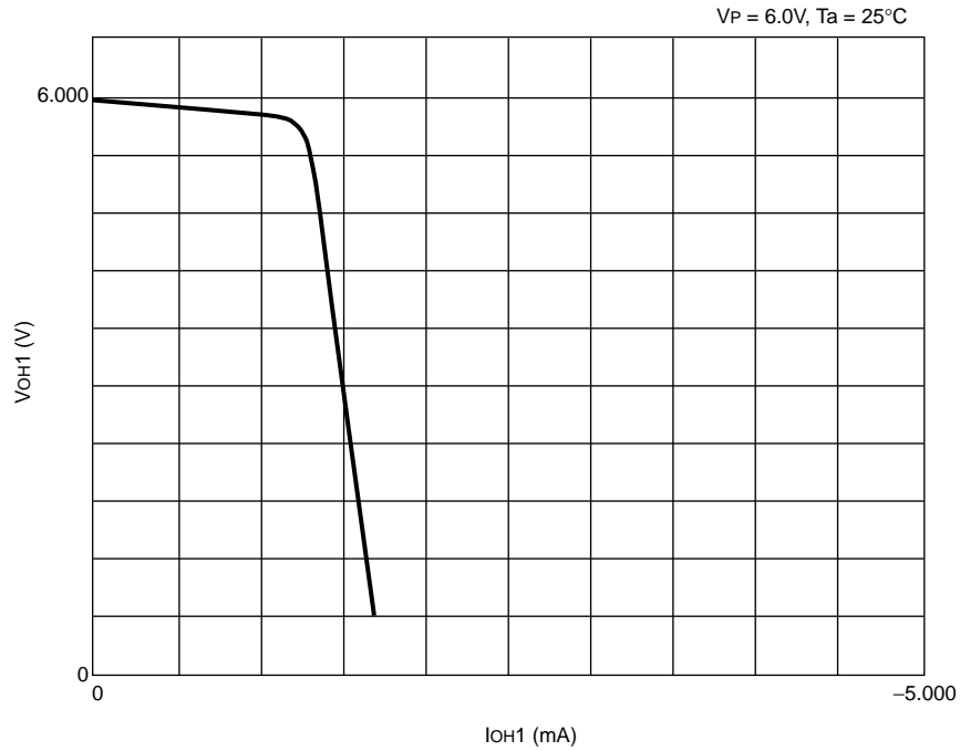
“H” level output current vs. “H” level output voltage (PLL2)
