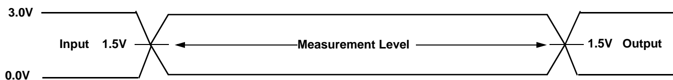
Figure 17. Input Waveforms and Measurement Levels
